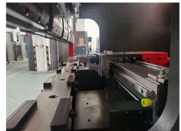
Z軸(突当上下) Y1/Y2軸(突当左右) Z Axis(UP/DOWN) Y1/Y2 Axis (RIGHT/LEFT)
